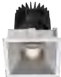
LED Power System Power LED Voltage LED Current CRI CCT Beam LED Output System Output Code 18 W 21 W 36 V 500 mA 90 2700K 24° 1900lm 1400lm SMS2G2-9272018N-WS 36° 1900lm 1400lm SMS2G2-9273618N-WS 45° 1900lm 1200lm SMS2G2-9274518N-WS 3000K 24° 2000lm 1500lm SMS2G2-9302018N-WS 36° 2000lm 1500lm SMS2G2-9303618N-WS 45° 2000lm 1300lm SMS2G2-9304518N-WS 4000K 24° 2200lm 1600lm SMS2G2-9402018N-WS 36° 2200lm 1600lm SMS2G2-9403618N-WS 45° 2200lm 1400lm SMS2G2-9404518N-WS 25 W 28 W 36 V 700 mA 90 2700K 24° 2400lm 2000lm SMS2G2-9272025N-WS 36° 2400lm 2000lm SMS2G2-9273525N-WS 45° 2400lm 1800lm SMS2G2-9274525N-WS 3000K 24° 2600lm 2100lm SMS2G2-9302025N-WS 36° 2600lm 2100lm SMS2G2-9303625N-WS 45° 2600lm 1900lm SMS2G2-9304525N-WS 4000K 24° 2800lm 2300lm SMS2G2-9402025N-WS 36° 2800lm 2300lm SMS2G2-9403625N-WS 45° 2800lm 2050lm SMS2G2-9404525N-WS 18 W 21 W 36 V 500 mA 90 2700K 24° 1900lm 1400lm SMS2G2-9272018N-WM 36° 1900lm 1400lm SMS2G2-9273618N-WM 45° 1900lm 1200lm SMS2G2-9274518N-WM 3000K 24° 2000lm 1500lm SMS2G2-9302018N-WM 36° 2000lm 1500lm SMS2G2-9303618N-WM 45° 2000lm 1300lm SMS2G2-9304518N-WM 4000K 24° 2200lm 1600lm SMS2G2-9402018N-WM 36° 2200lm 1600lm SMS2G2-9403618N-WM 45° 2200lm 1400lm SMS2G2-9404518N-WM 25 W 28 W 36 V 700 mA 90 2700K 24° 2400lm 2000lm SMS2G2-9272025N-WM 36° 2400lm 2000lm SMS2G2-9273525N-WM 45° 2400lm 1800lm SMS2G2-9274525N-WM 3000K 24° 2600lm 2100lm SMS2G2-9302025N-WM 36° 2600lm 2100lm SMS2G2-9303625N-WM 45° 2600lm 1900lm SMS2G2-9304525N-WM 4000K 24° 2800lm 2300lm SMS2G2-9402025N-WM 36° 2800lm 2300lm SMS2G2-9403625N-WM 45° 2800lm 2050lm SMS2G2-9404525N-WM
